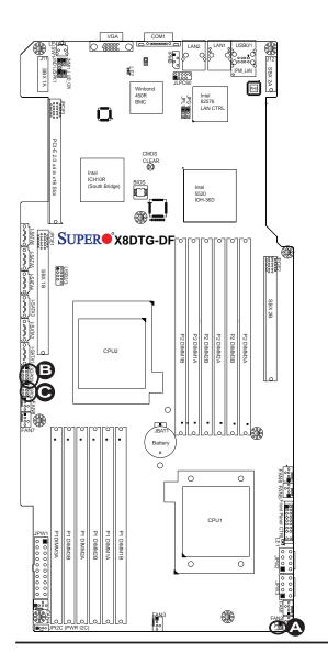
A. Chassis Intrusion B. T-SGPIO0 C. T-SBPIO1
